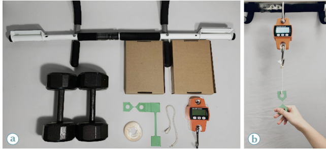
Figure 15: (a) Equipment needed for mechanical testing with our toolkit. (b) At-home setup for performing tensile strength mechanical tests using our toolkit.
