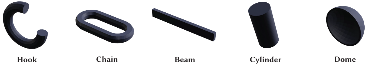
Figure 13: The five primitive geometries used in our evaluation: hook, chain, beam, cylinder, and dome. Each represents a distinct load condition relevant to structural 3D prints.
